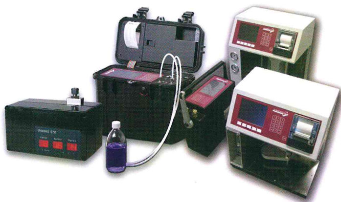
Equipped with eight or more size channels, automatic particle counters are able to detect bearing failures in lubricating oil systems at an early stage
