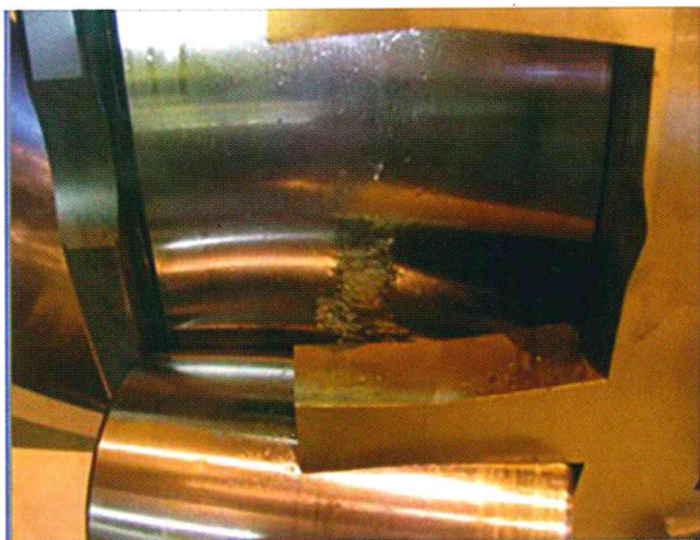
Defective roller bearing in a Finnish paper mill
