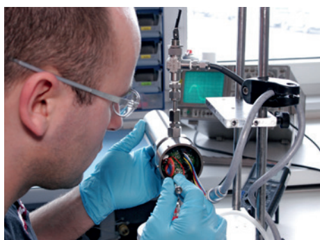
The PAMAS After Sales Service can be booked also on site: For this purpose, specially trained service engineers directly come to the customer's place bringing along the equipment which is required for the standardised calibration of automatic particle counters. (Picture: PAMAS)
