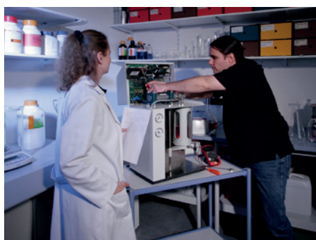
In order to assure constant measuring accuracy, automatic particle counters must be recalibrated at least once a year. PAMAS offers an After Sales Support for calibration and repair. This service may also be combined with a Service Contract. (Picture: PAMAS)
